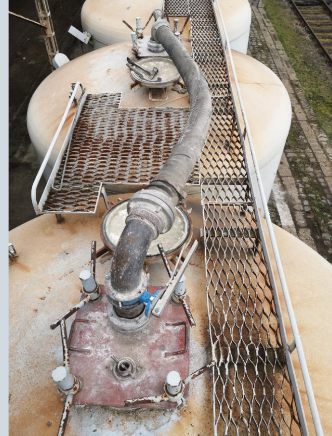
D, FIT THE FLEXIBLE MATERIAL PIPE
